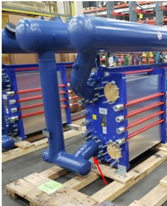
Figure 5. Drop leg on flooded evaporator. Red arrow indicates the dropleg [2].
