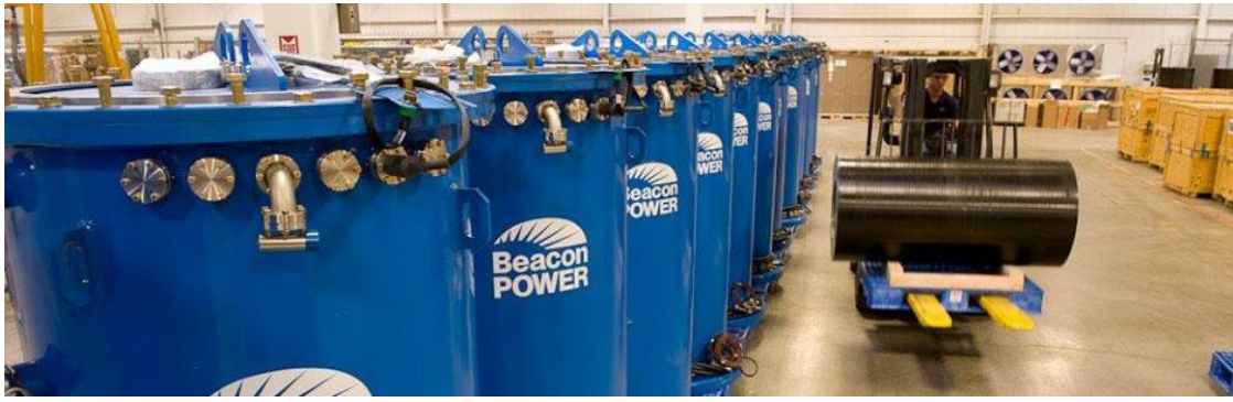
Figure 29: Photo of Beacon Power’s flywheels [6]. The fiber composite flywheel itself is seen to the right on the fork-lift. Each unit is 100 kW. Photo from manufacturer’s store.
