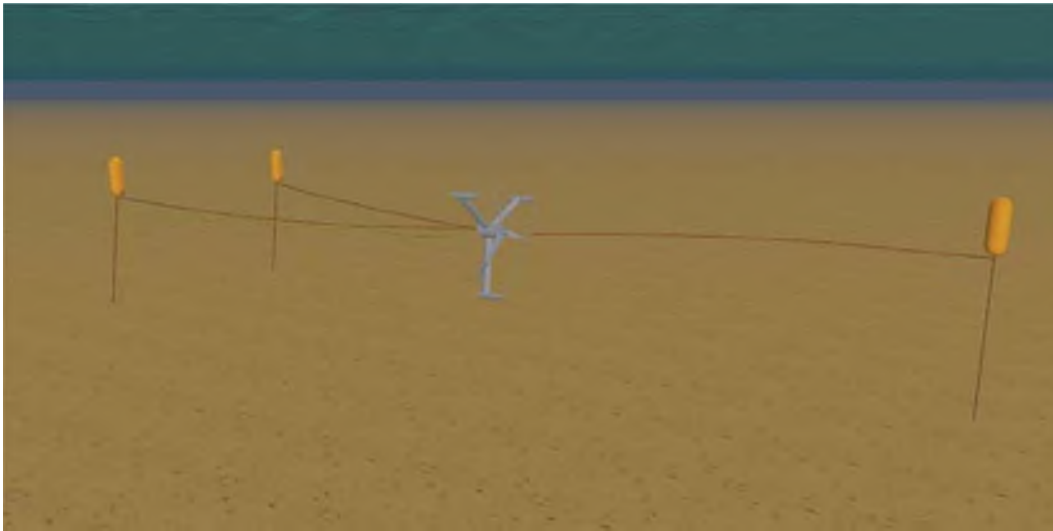
Figure 64: Foundation types: Second generation devices - Mooring system based on wires and buoys.[7]
